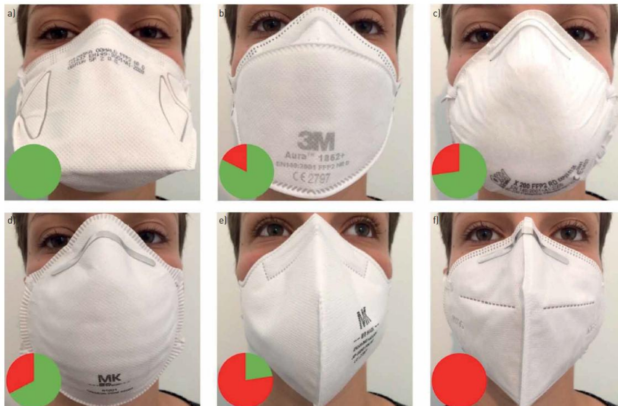
FIGURE 1 Different respirators evaluated by fit testing for tight sealing of nose and mouth. a) Polmaska Donald; b) Aura 1862+; c) X200; d) AP-81001; e) AP-83001; f) KN95 type. Pie charts show the percentages of tight sealing (green) and nonsealing (red) respirators in healthcare workers.
